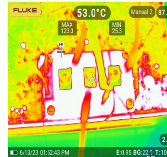
IGBT open module under test
